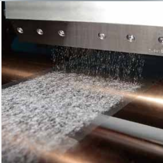
Curtain spray coating
