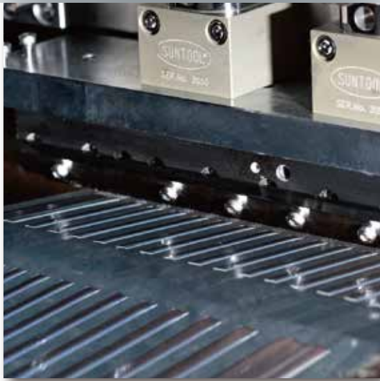
Coating process by slot die coater
