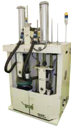
(Barrel-shaped melt adhesive applicator 088 for cylinder use)
